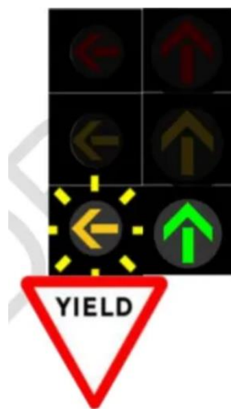
Figure 39: Suggested 'Mini-Yield' Sign for use with Flashing Amber Arrow
