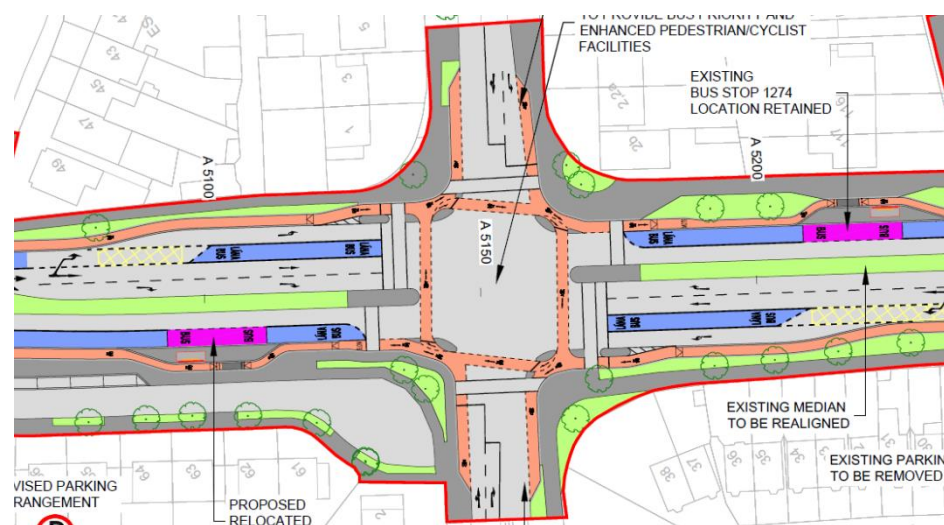
Figure 25: BusConnects Junction Type 2 example
