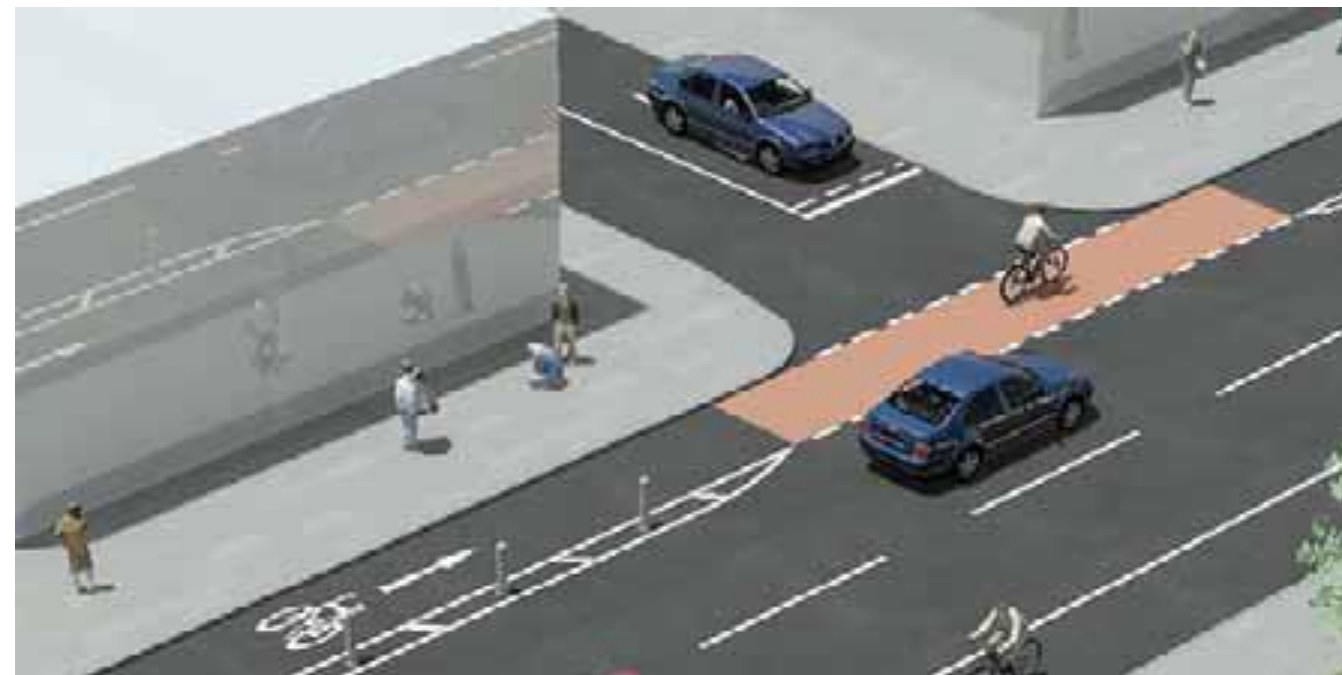
Figure 32: On-Road Cycle Lane Priority Junction Treatment
